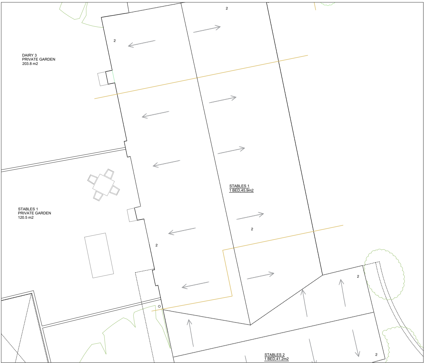
Proposed Roof Plan - Stables 1 1:100
